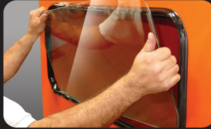
2. Lubricate Locking Gasket. Then slide glass in bottom first.
