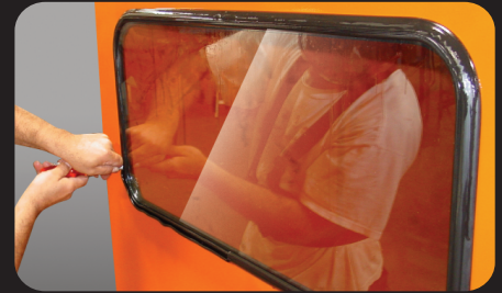
3. Finish working rubber around glass with tools found on pages 44-45.
